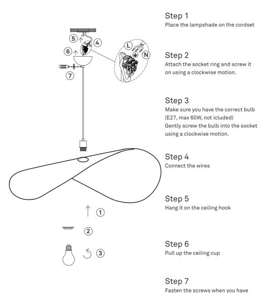
adjusted the cable to desired length.
